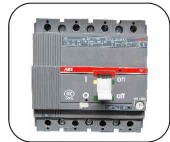
Four pole MCCB in accordance with AS3010. The motorised MCCB is fitted with a stunt trip to protect the generator in event of a sudden shutdown.
