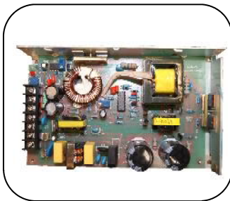
Dedicated battery charger with boost and flat modes. Battery charger is configured to provide an alarm in event of a fault with the charging system.
